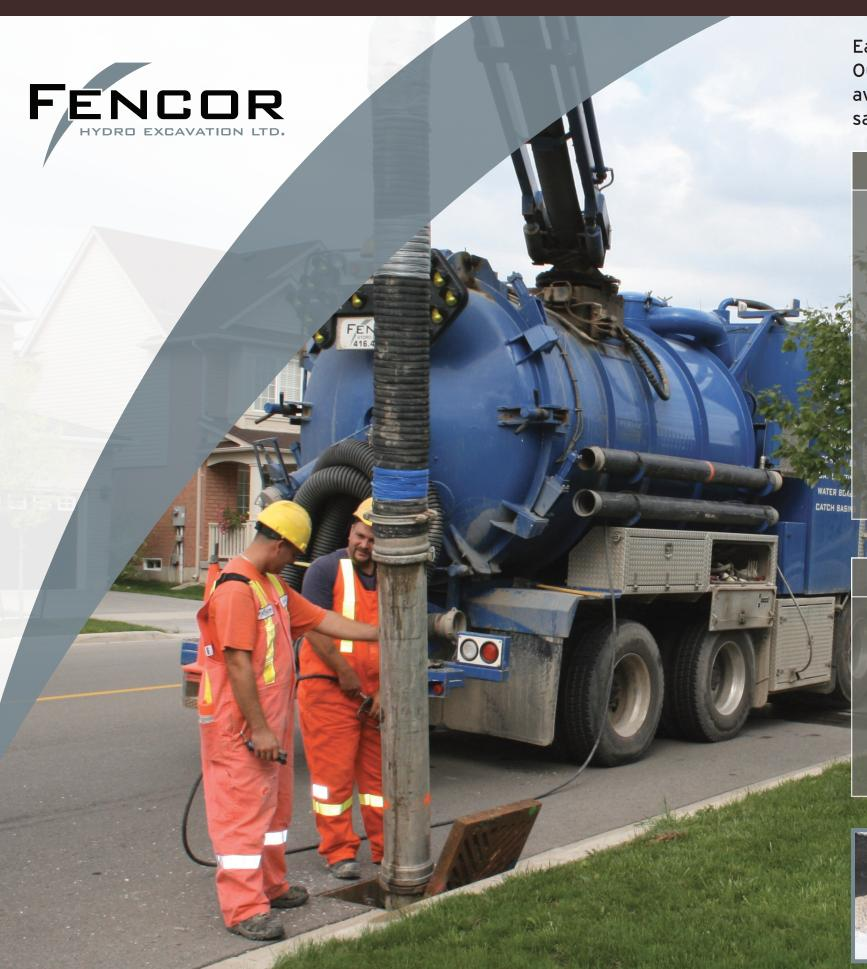
Each truck in our fleet is equipped with industry leading technology. Our 6400 CFM Vacuum accompanied with 6000 psi water displacement and available diesel powered hot water heater, allow us to efficiently excavate safely regardless of weather or frozen ground.
